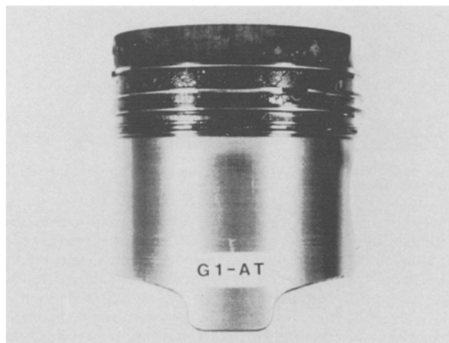
FIG. 10. Carbon buildup on the piston after the durability test with the microemulsion.
